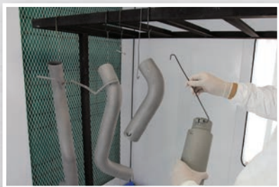
Racking Exhaust Pipes
