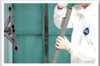
Racking Exhaust Pipes
